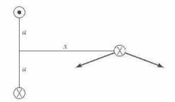
b) If the wire carries current out of the page then the forces felt will be the opposite of part (a). Thus the force will be  $1.11 \times 10^{-5}$  N/m, upward.
